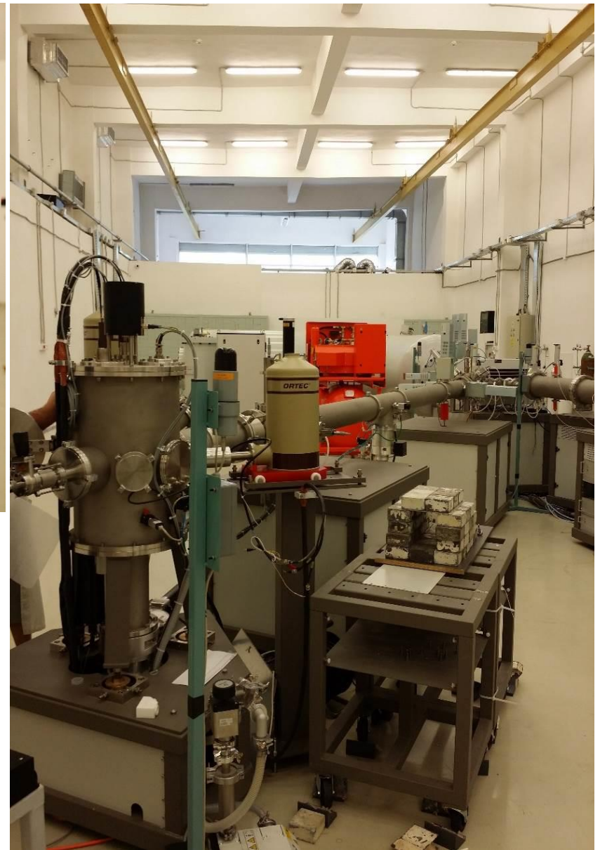
PIXE-PIGE-RBS analysis system at nuclear tandem accelerator in Bucharest-Magurele
